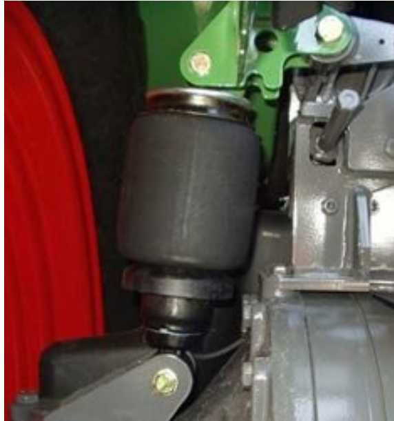
Figure 8. The air spring shock absorber. (courtesy: Fendt tractors)
