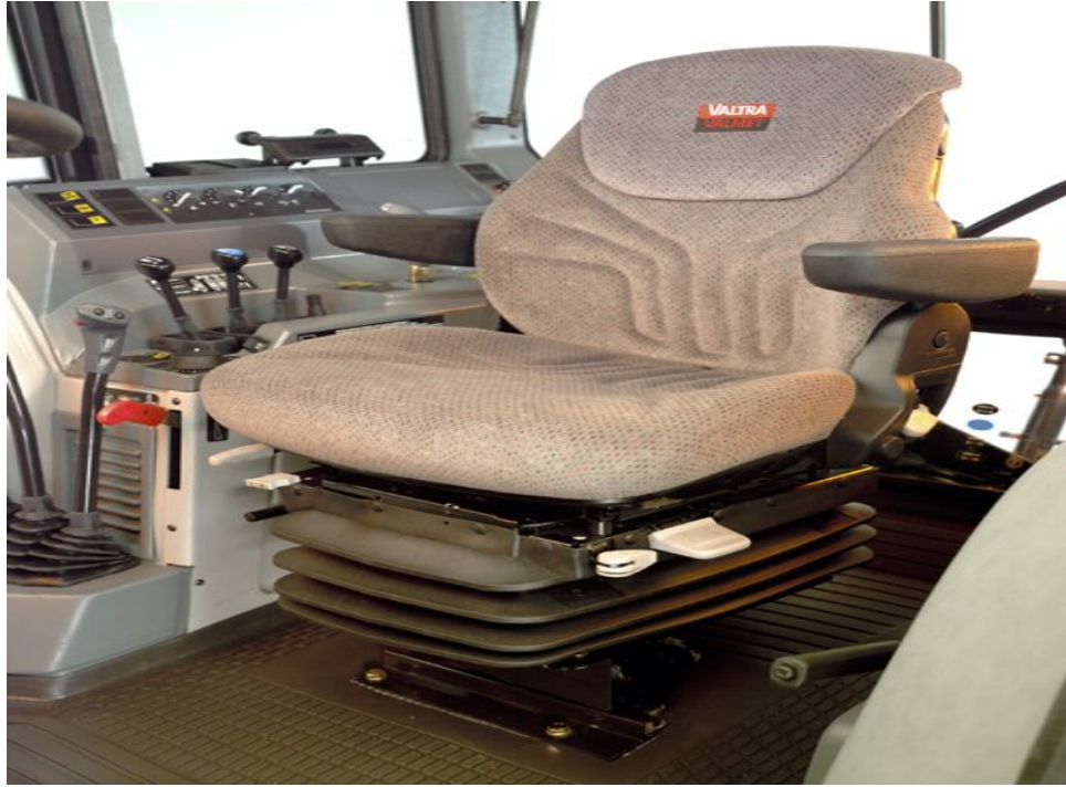
Figure 12. A Valtra seat with Positive Response air suspension system. (courtesy: Valtra tractors)
